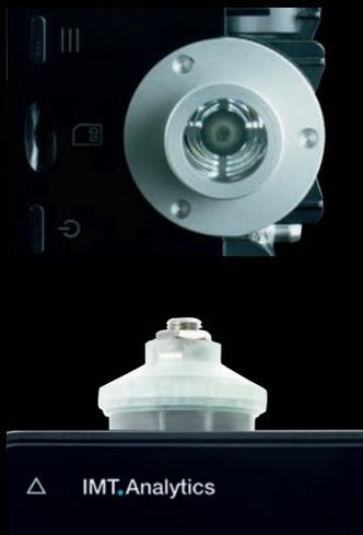
CITREX H3 can measure the key ventilation parameters. The measuring instrument is also ideal for flow and pressure measurements. Since gas standards and gas types can be set to suit requirements, CITREX H3 is highly flexible in use. The extremely compact and light instrument offers everything you need to verify home ventilators and intensive care ventilators.
