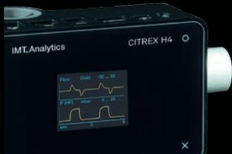
CITREX H4 is designed for mobile and effortless application, meeting all the requirements of daily use in the field. Its numerous functions make it possible to subject various medical devices to advanced performance testing. CITREX H4 is suitable for checking ventilators, anaesthetic machines, oxygen blenders and suction equipment.
